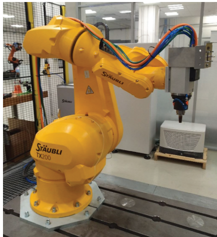
Figure 1. Industrial robot with 6 joints.
