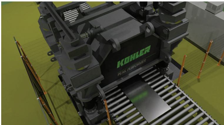
Figure 3. The digital twin of the roller levelling process in a virtual environment.
